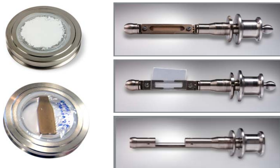
Figure 2: Practical examples of sample preparations (powder, solid sample and liquid sample)
