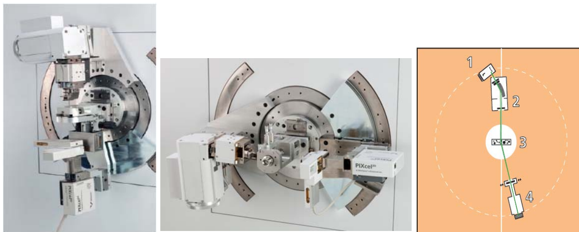
Figure 1: Schematics and photographs of experimental SAXS setup: 1: X-Ray tube. 2: beam defining slits and X-ray mirror, 3: sample stage, 4: anti-scatter slit and detector
