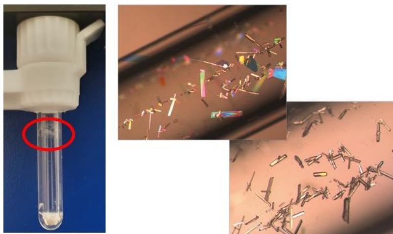
Rys. 1. Salicylamide crystals grown by sublimation in CrystalBreeder.
