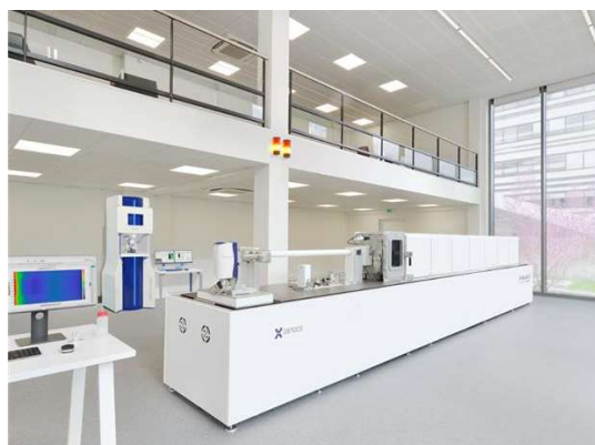
Fig. 1. Xeuss Pro horizontal platform for SAXS/WAXS/GISAXS/USAXS and imaging alongside the Nano-inXider compact vertical system.
